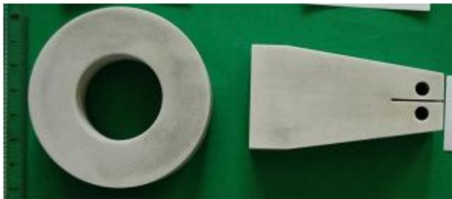
**Figure 3.1.** Two samples that have been used to generate fracture surfaces of glass ceramics: modified Brazilian test geometry that leads to rapid mode I fracture (left) and modified Tapered Double Cantilever Beam geometry that leads to stable mode I fracture (right). The outside diameter of the annular sample is 80 mm.
