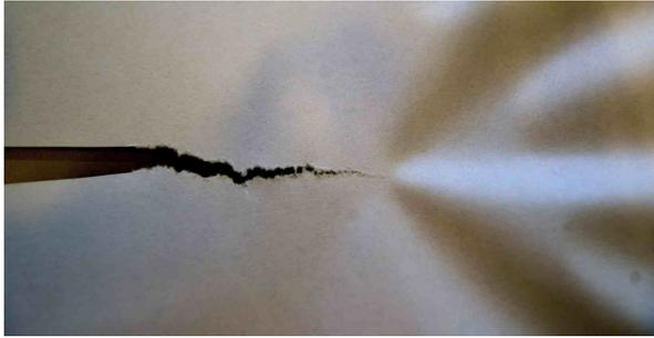
**Figure 3.1** A crack propagating in paper. The crack emerging from the straight notch is rough to the eye. One can also distinguish a large damaged zone where the crack is partially closed at some points. Although the material can be considered as two-dimensional, the loading conditions are 3D, as evidenced by the out-of-plane displacement of the sheet, visible on the picture.
